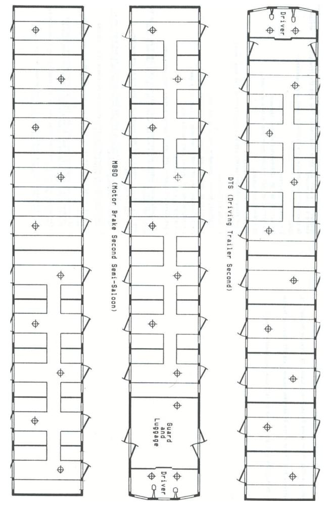
**Internal configuration of EPB units:** 2EPB comprises 1x MBSO and 1x DTS.
